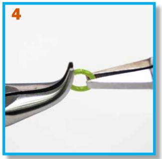
When closing the ring, bring the left and right sides together, making sure to leave no gap between the two. Align the ends as close as possible.
