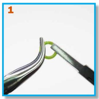
To open a ring, use 2 sets of pliers and grab the ring on the left and right sides.
